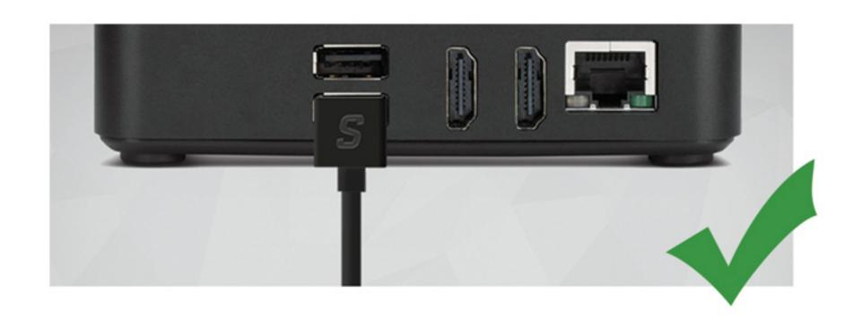
Always connect the Usb-Progammer directly to the usb port of your PC.
